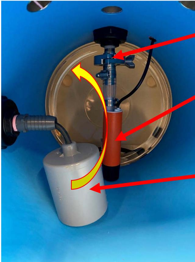
Pump quick-release fasteners
