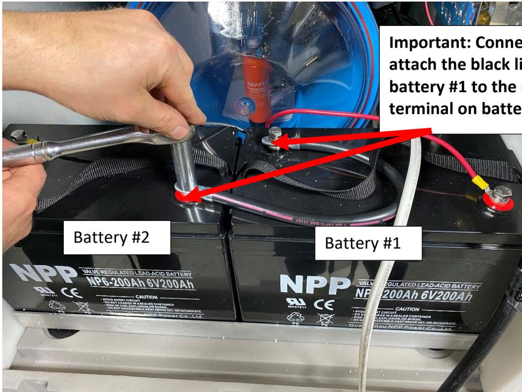
**Important: Connect and attach the black line of battery #1 to the red terminal on battery #2.**
