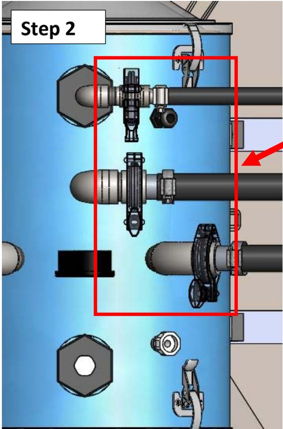
Unscrew and remove the quick-release fasteners, taking care not to lose the silicone gaskets.
