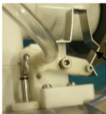
As the sap level goes down, The float also goes down, the Spring keeps the rocker arm up and the vacuum on the right side of the cylinder
