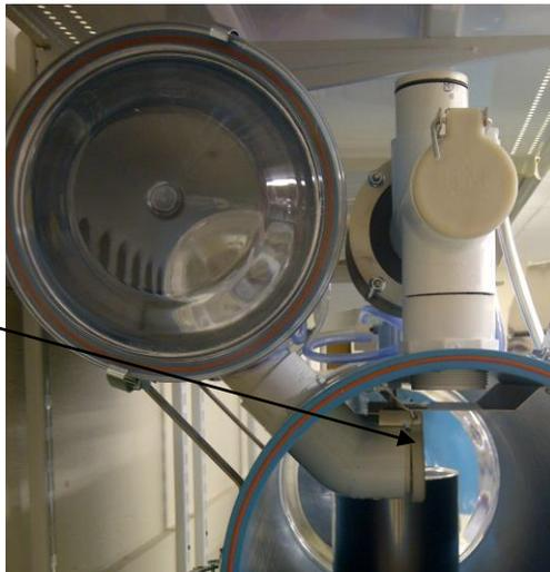
When the releaser dumps, the vacuum left in the tubing system and the manifold shuts down the doors in the releaser. The sap will accumulate in the manifold until the floats goes back down and releases
