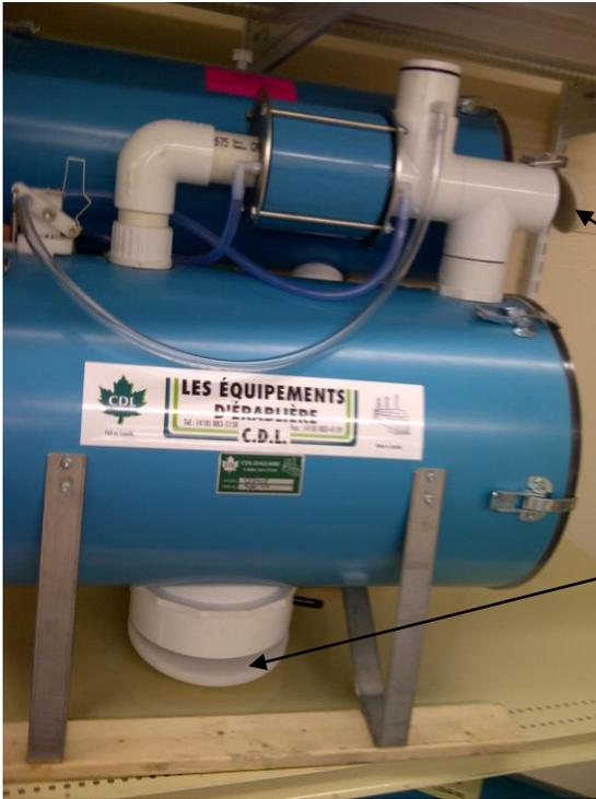
When the cylinder rod shifts to the right, it opens the cylinder cap, releasing vacuum from the
