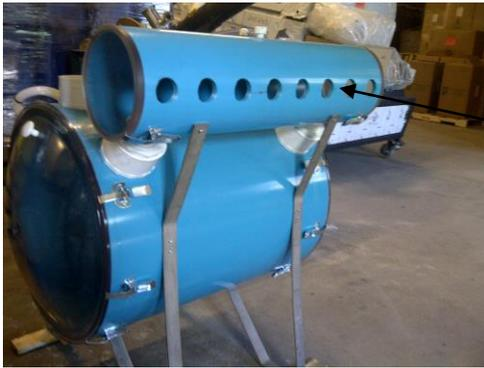
The wet and dry lines will come in the back of the manifold in the pre-drilled holes
